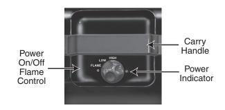
**ROTARY POWER ON/OFF FLAME CONTROL:** This heater has two heat settings: HIGH and LOW. Use the higher setting (1200 watt) to raise the room temperature quickly. When the desired temperature is reached use the LOW (600 watt) setting. It is usually sufficient to maintain a comfortable temperature.
