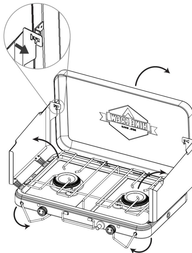
2. Lift the grill grate and remove the regulator from its storage.
