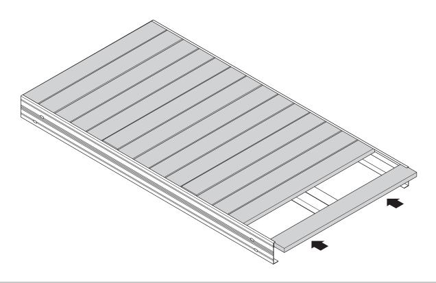
9 Fit one end of the remaining End Rail into the Side Rail (9a). The End Rail fits in between the flanges on the Side Rail (9b).
