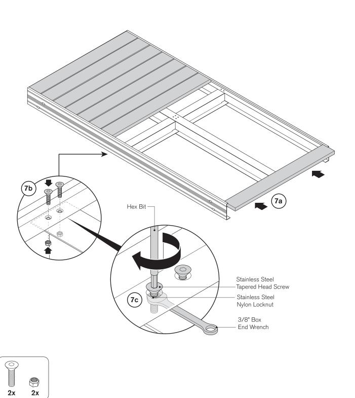
Install the remaining deck boards into the frame.
