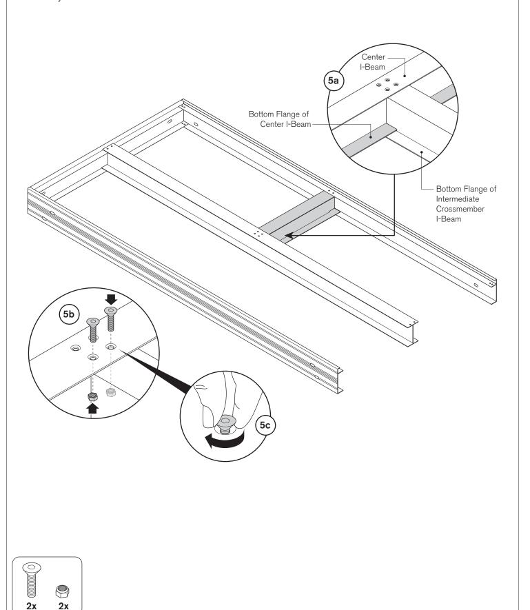
You now have all the frame components attached to the frame except the last End Rail. Make sure all of the connections are fitted tightly and tighten all of the screws you have installed so far on the top side of the frame. Use the Hex Bit to fully tighten the Stainless Steel Tapered Head Screw while holding in place the Stainless Steel Nylon Locknut with a 3/8" Box End Wrench.
