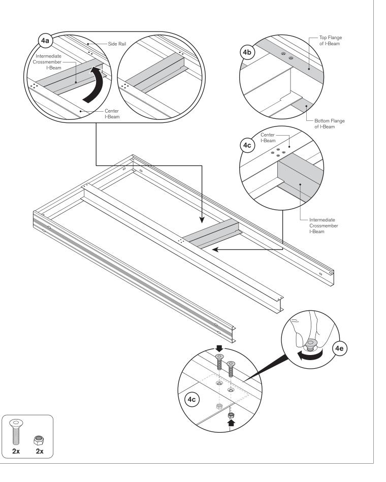
Notice that the bottom flange of the Intermediate Crossmember I-Beam fits underneath the bottom flange of the center I-Beam (5a). Insert the screws and lock nuts (5b) and hand tighten (5c). Attach the second Crossmember in the same manner as the first, but do not install the screws into this side rail yet.
