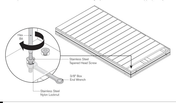
Use the Hex Bit to fully tighten the Stainless Steel Tapered Head Screw while holding in place the Stainless Steel Nylon Locknut with a 3/8" Box End Wrench.
