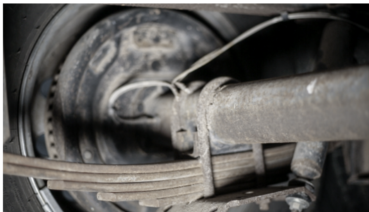
FACTORY GAP BEFORE TRAILER SUMOSPRING INSTALLATION
