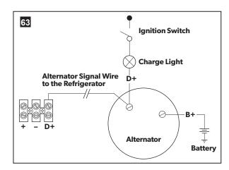
➤ Connect the vehicle's alternator (D+) to the D+ on the terminal block
