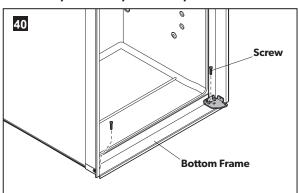
➤ Secure the refrigerator using two screws (not provided) through the bottom frame of the refrigerator.
