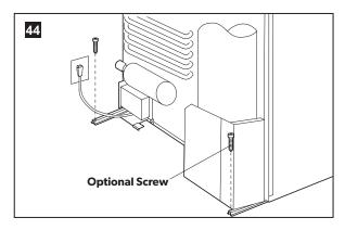
➤ Install one screw (not provided) in the rear base. An optional screw may be added on the opposite side.
