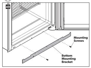
➤ Open the fresh food door and secure the bottom mounting bracket to the refrigerator using the screws provided.
