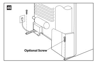
➤ Install one screw in the rear base. An optional screw may be added on the opposite side.
