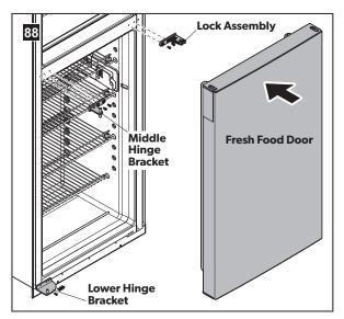
To reinstall the fresh food door, lock, and middle hinge bracket, do the following:
