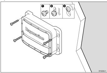
**Note:** Drill bit, tap size and tightening torque is dependent on the thickness and type of material the unit is to be mounted on.
