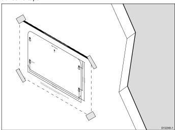
2. Drill 4 holes at the marked location on the template.
